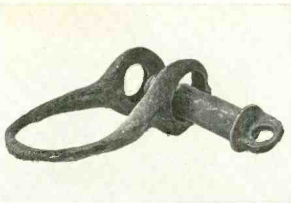
Formerly galvanized shackle was connected to a stainless-steel mooring pennant for one season—blamed on technician.
